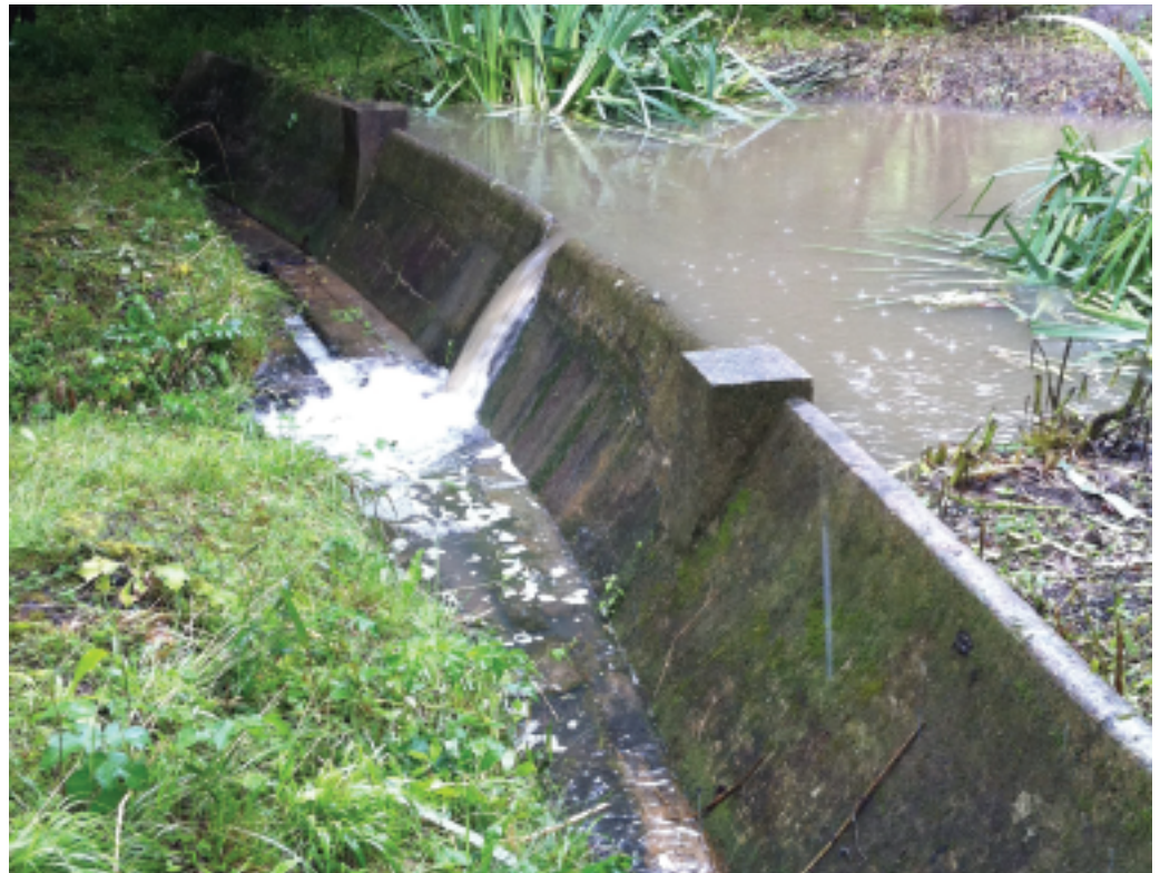
The gap in the dam: The scale model of the breached Möhne dam used in wartime testing
